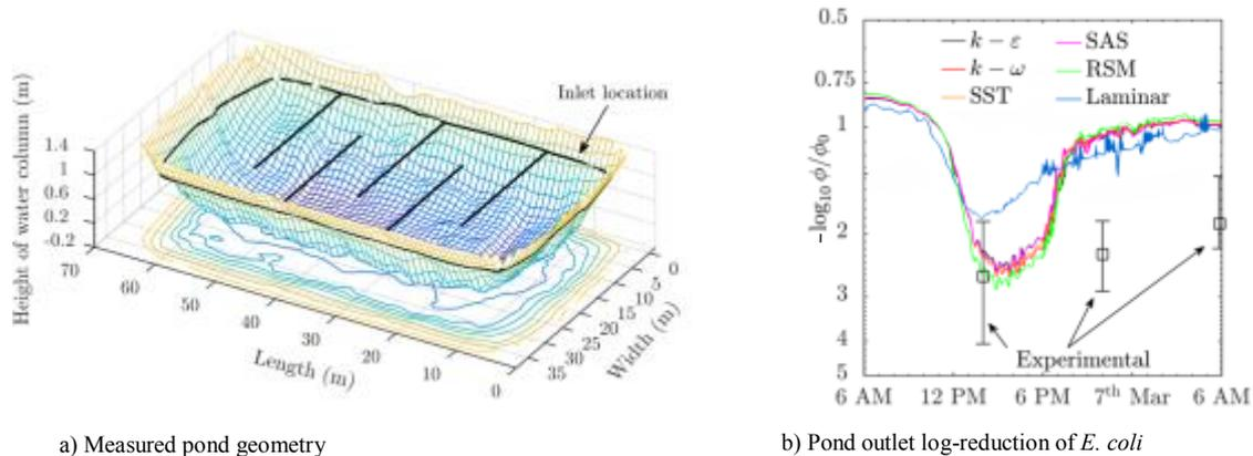
Fig. 1. a) Measured geometry of the maturation pond - the water-level and baffle placement are shown by dark solid lines. Note that the depth scale is exaggerated; b) Measured and predicted outlet surface concentrations of *E. coli* for 6/7<sup>th</sup> March 2015.
