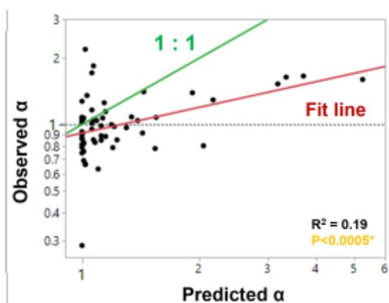
**Figure 2.** Observed chemical enhancement factor ( $\alpha$ , dimensionless) versus that predicted from the theoretical model of Hoover and Berkshire (1969). If the model fits well, the dots should be close to the green line.
