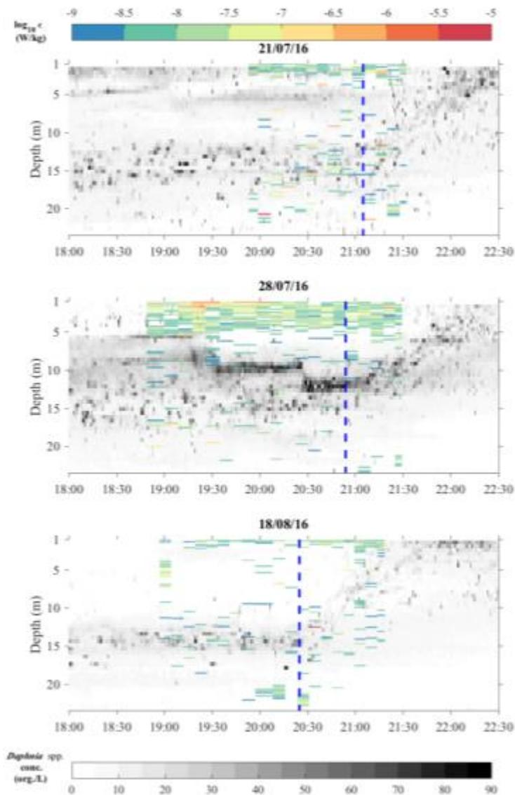
Figure 1: TKE dissipation rates  $\epsilon$  in the foreground (top colour-bar) overlapped with the estimated *Daphnia*'s concentration (bottom grey colour-bar). Blue dashed line shows the sunset time when DVM begins.
