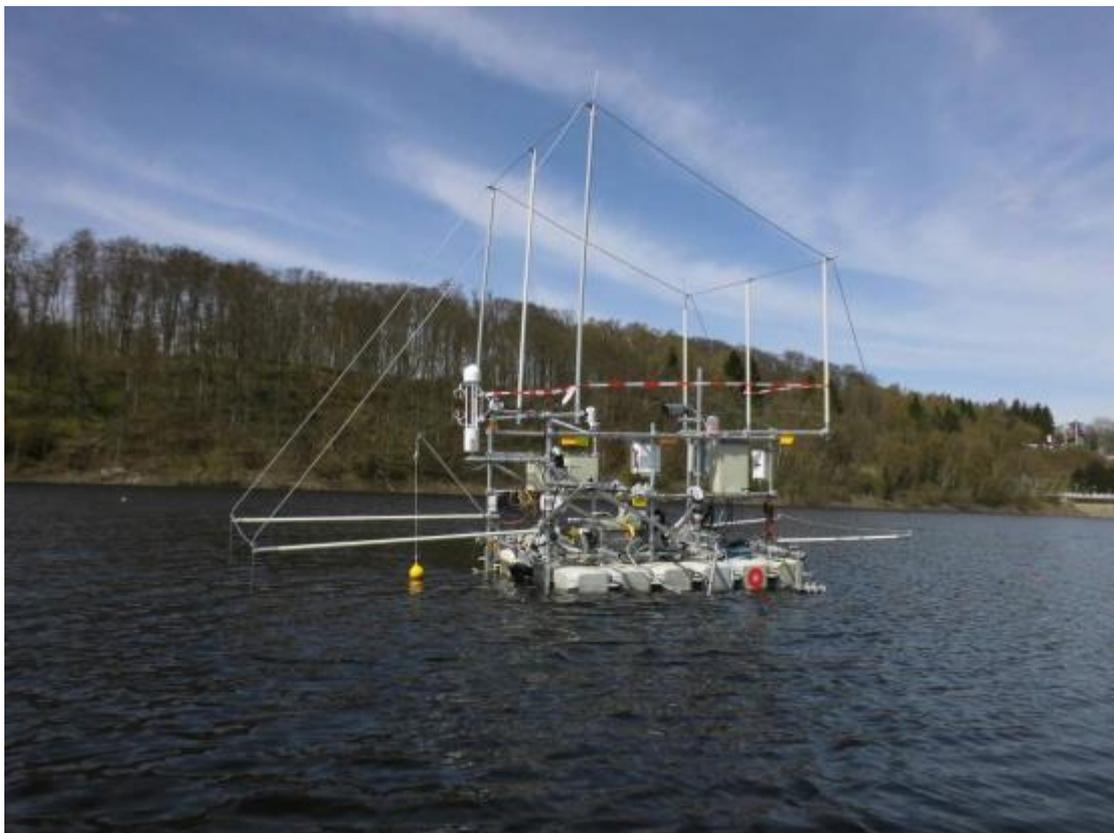
**Figure 1:** Floating micro-meteorological and hydro-chemical measurement station on Rappbode reservoir in Harz Mountains. The poles and wires are for lightning protection.
