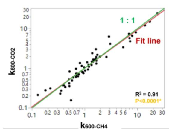
**Figure 1.** The relationship between the gas exchange velocity ( $k_{600}$ ,  $\text{m d}^{-1}$ ) estimated from  $\text{CO}_2$  and  $\text{CH}_4$ . Green line and red line represent line of equality and regression fit, respectively.
