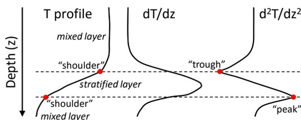
**Figure 1: Layer-identification process (repeated at multiple scales)**
