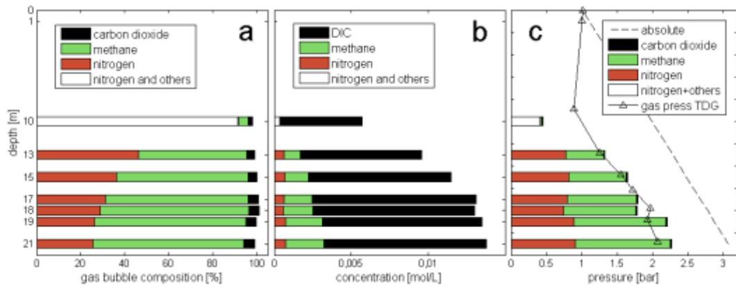
Fig. 1. (a) Measured gas concentration in the gas bubble of samples versus depth (b) calculated gas concentration in the lake (c) gas pressures based on gas concentration compared with direct gas pressure measurements (from [2]).
