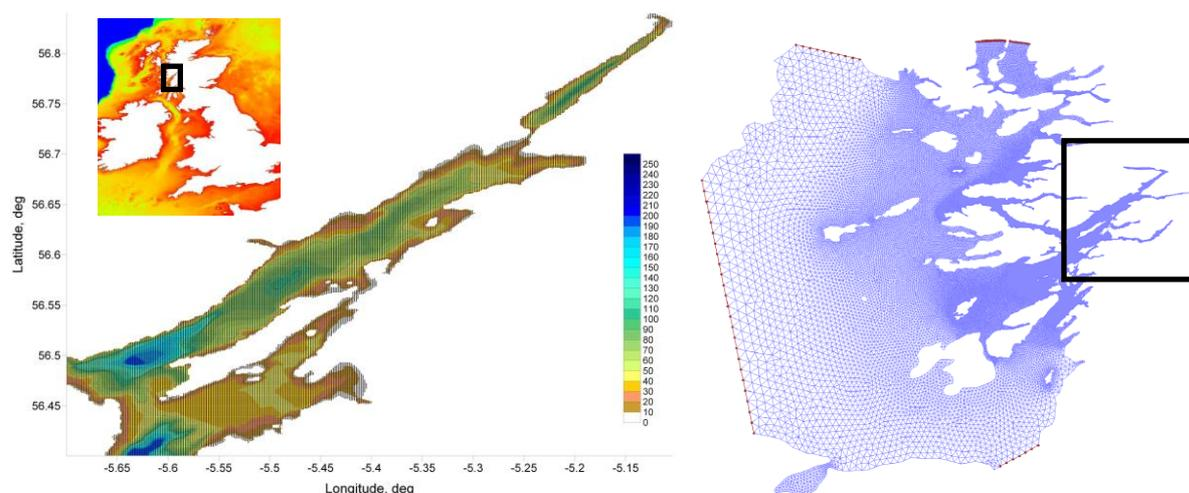
Figure 1: Left: POLCOMS Loch Linnhe model bathymetry (no side lochs resolved). Small map shows location of Loch Linnhe. Right: FVCOM model grid showing the larger extent of this case study and Loch Linnhe (including side lochs) in the black box.
