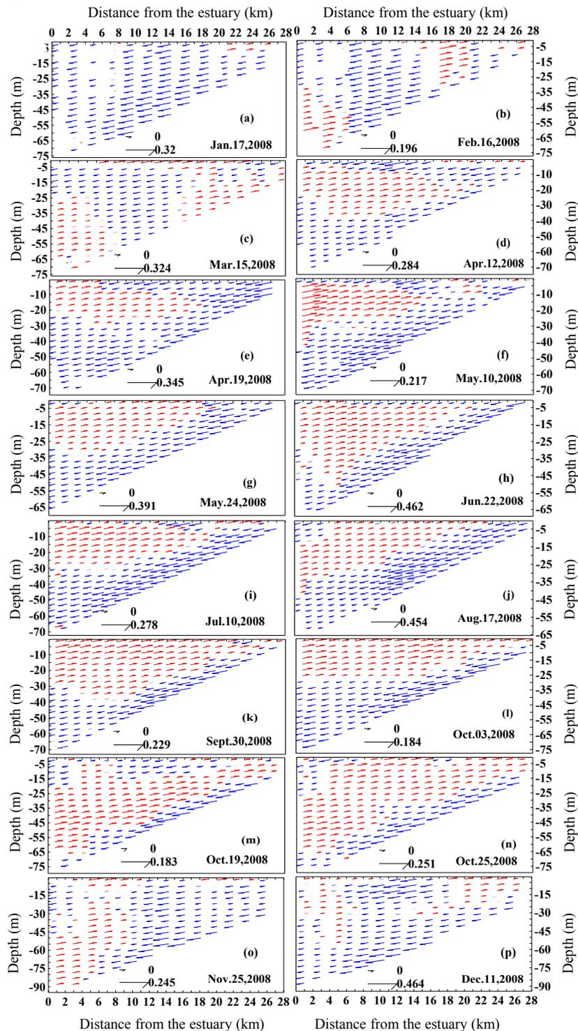
Fig. 3 Longitudinal-vertical velocity profile of the Xiangxi Bay in 2008 (Unit: m/s)
