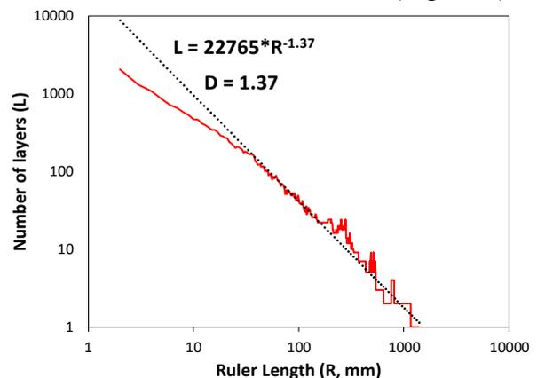
Figure 3: Example of a profile pseudo-spectrum, showing increase in number of layers ( $L$ ) in profile with decrease in resolution scale (ruler length,  $R$ ) and best fit power law line with fractal dimension  $D$
