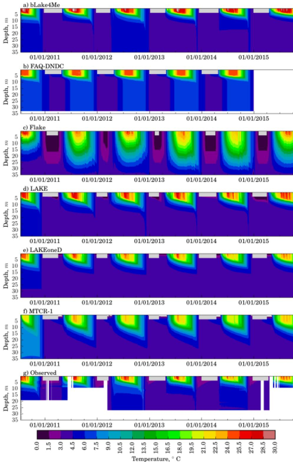
Fig.1. Time-depth profiles of temperature in Harp Lake, reference model run and observation data. The grey boxes indicate duration of the ice-cover period, the white patterns - a lack of data
