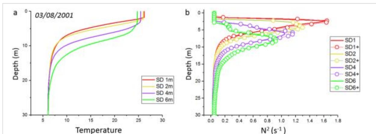
**Fig. 1** Lake Hallwil top 30 meters on 3 August 2001. a) Temperature profiles at increasing water transparency. b)  $N^2$  profiles for increasing water transparencies (solid line) and for the same at an air temperature increased by 2°C over the analysed period (April-December 2001).
