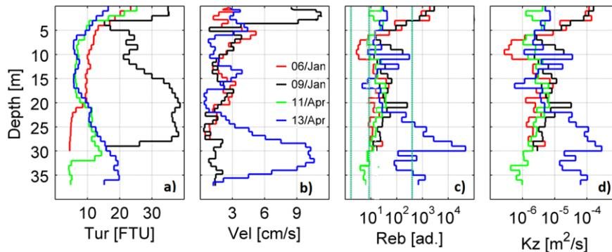
**Figure 2.** Bin and time averaged profiles (1 m bin per day) of a) turbidity, c) velocity (no velocity April 11), d)  $Re_b$  (green vertical lines define turbulent regimes according to BB) and e) vertical eddy diffusivity.
