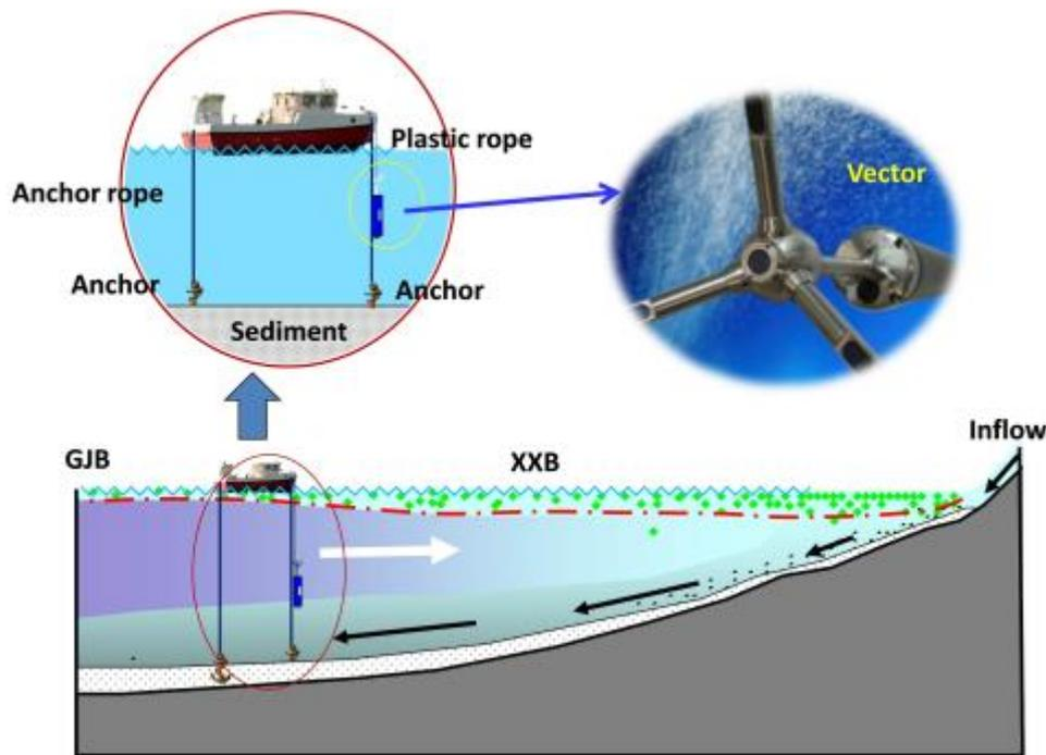
Fig. 2 Schematic diagram of field monitoring of velocity (Ma et al., 2011)
