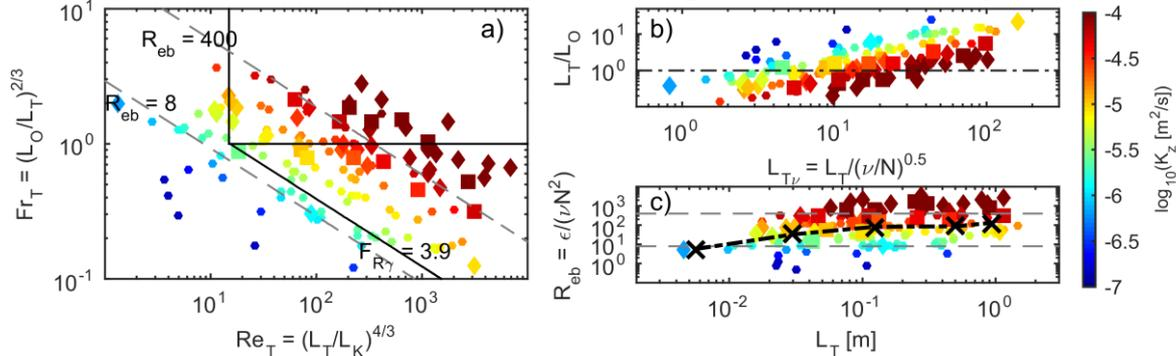
**Figure 3.** a)  $Fr_T$ - $Re_T$  diagram and limits by following I&I, b) The ratio  $L_T/L_O$  as a function of  $L_{Tv}$  (Mater et al, 2015) and c)  $Re_b$  as function of  $L_T$ . Gray dashed lines in a) and c) mark the  $Re_b$  regimes and in b) the ratio  $L_T/L_O = 1$ . In the figures the rectangles mark the plume zone in April 13 (below of 23m), diamonds the mixing zone (above of 4m) and the circles the remaining data. Black cross-dashed line in c) is a running mean of  $Re_b$ .
