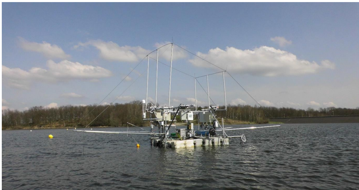
Figure 1: Floating observation platform installed on the Bautzen reservoir and equipped with micrometeorological and hydro-chemical measurement systems for continuous monitoring of mass- and energy exchange between water surface and atmosphere
